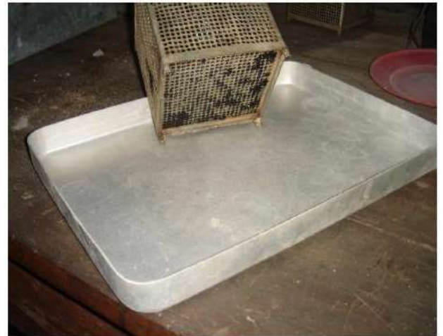
Fig 8: No drain down in case of sample with fiber
