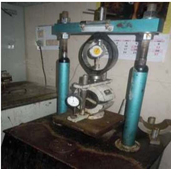
Fig 7: Marshall test being conducted with the Marshall apparatus.
