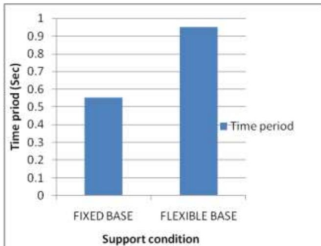
**Fig 7:** Time period (Sec) for fixed base and Flexible base infill frame model
