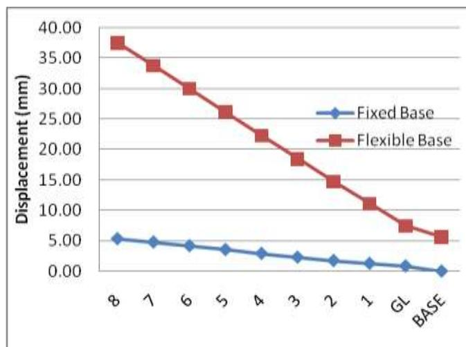
**Fig 5:** Displacement (mm) at different stories between fixed base and flexible base infill model.
