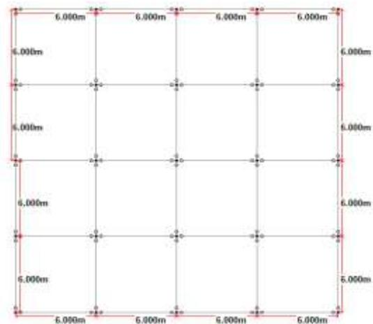
**Fig -1:** Plan of infilled building frame model
