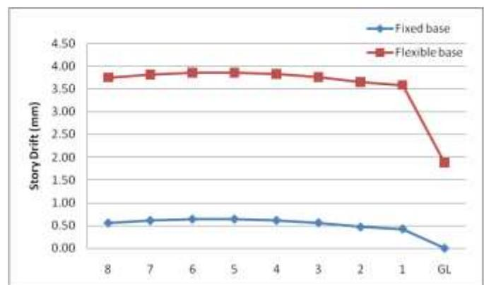
**Fig 6:** Story Drift (mm) at different story between fixed base and flexible base infill frame
