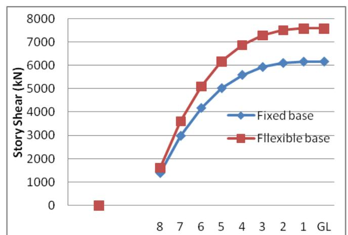
Fig -4: Story shear (kN) at different story for fixed base and flexible base infill model.
