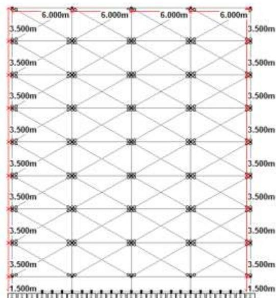
**Fig -2:** Elevation of infilled building frame model
