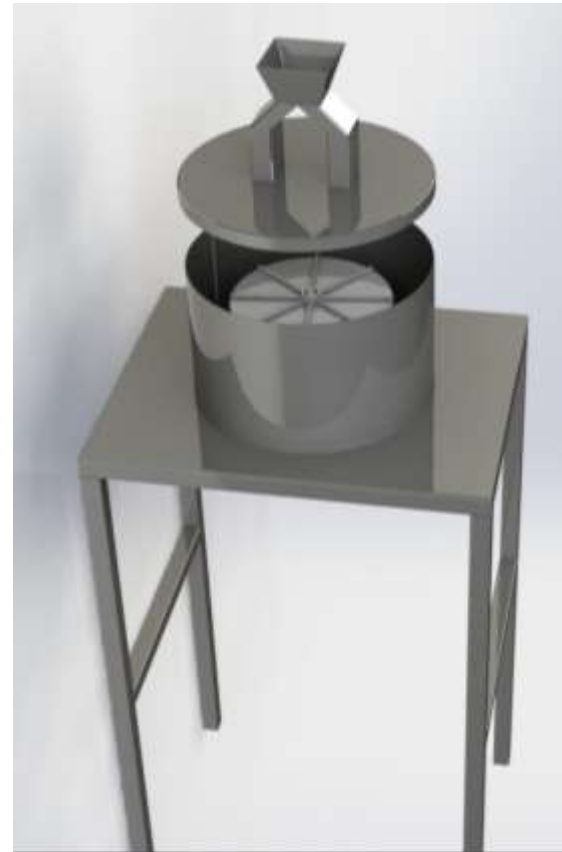
Fig. 1: Automatic Scooping Machine ( CAD Model )
