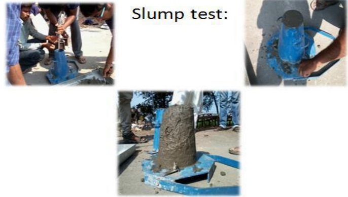
Fig-4: Slump Cone Test
