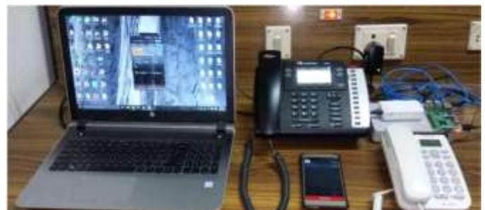
Fig -12: Hardware set up of Proposed IP-PBX system
