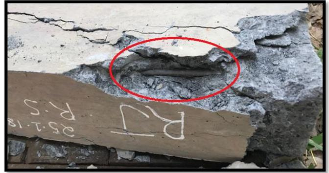
Fig -4: Cover failure and reinforcement exposure of rebar specimens
