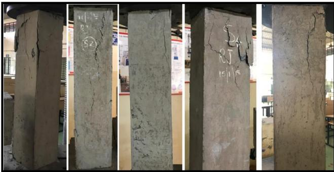
Fig -2: Crack pattern PCS square specimens
