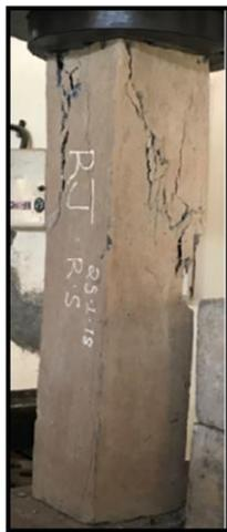
Fig -3: Crack pattern rebar specimen
