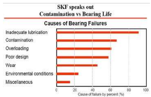
Fig. - 1 Causes of bearing failure
