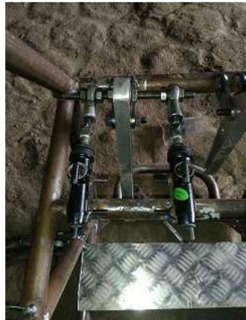
Figure 11 - Brake pedal Assembly
