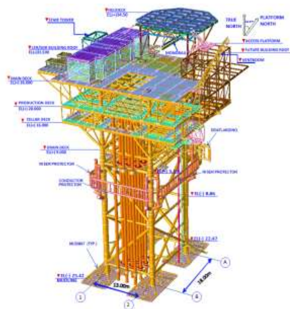
Figure-2.1.1 3D View of the Wellhead Platform
