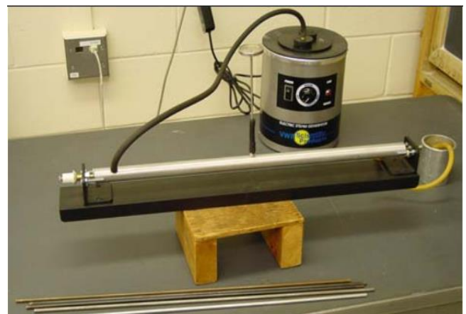
Fig – 1: The linear expansion apparatus. The rods are placed inside the silver jacket and the whole assembly is placed o the black base.
