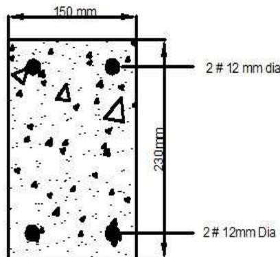
Fig 2: Cross sectional view of the beam weak in Flexure
