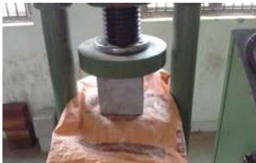
Fig 5: Testing of Cube in CTM
