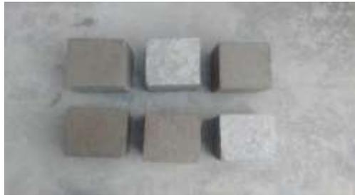
Fig 3: Conventional Concrete cube
