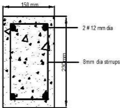
Fig 1: Cross sectional view of the beam weak in Flexure
