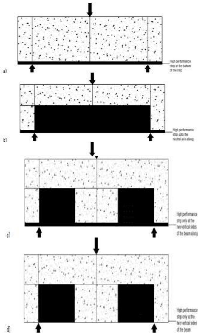
**Fig: 12. a) Strip placed on the soffit of the beam**
