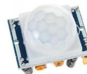
Fig -3.4:Motion Sensor
