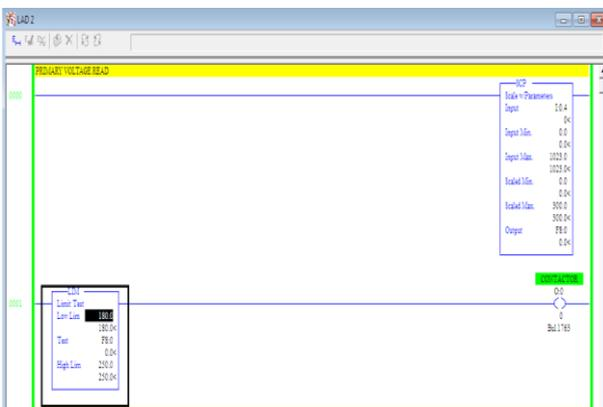
Fig -4: Real time value of primary voltage.
