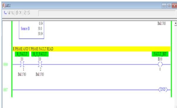
Fig -3: Protection against phase to phase fault.
