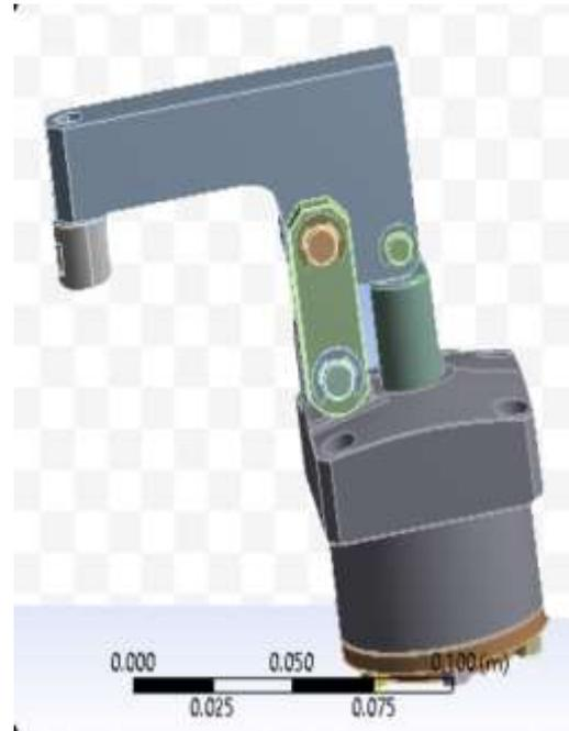
Fig.3 (i): Cylinder clamp assembly
