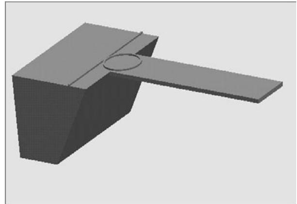
**Fig -1** : Schematic diagram of the cantilever integrated with the micro ring resonator.  $l$ ,  $t$  and  $w$  represent the length, thickness and width of the cantilever, respectively.
