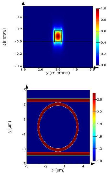
**Fig -4** (a) Mode profile of quasi-TE0 (b) Effective index of Micro ring Resonator
