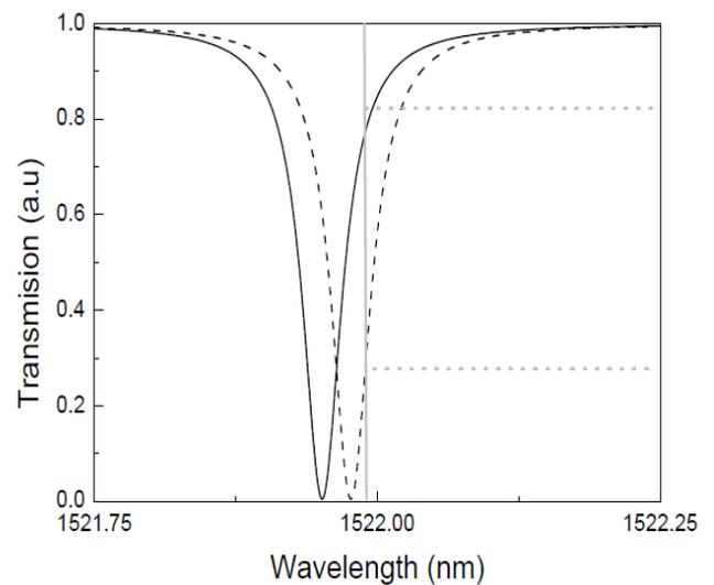
**Fig -3:** Sensor concept based on a ring resonator. The optical power modulation takes place as position of resonance dip shifts. Inset shows the variation of the output intensity
