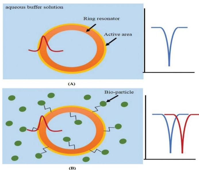
**Fig -2:** Optical ring resonator as a biological sensing platform; (a) ring resonator is placed in an aqueous buffer
