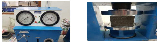
Fig 2: Compressive Testing Machine and Specimen Placed in Machine
