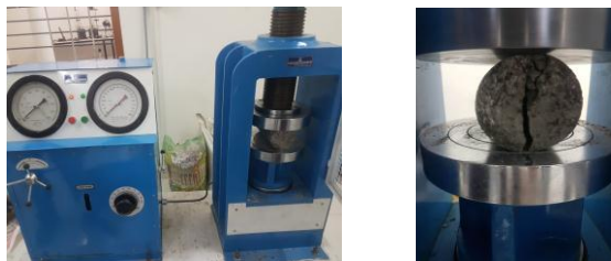
Fig 3: Split Tensile Testing Machine and Specimen Placed in Machine
