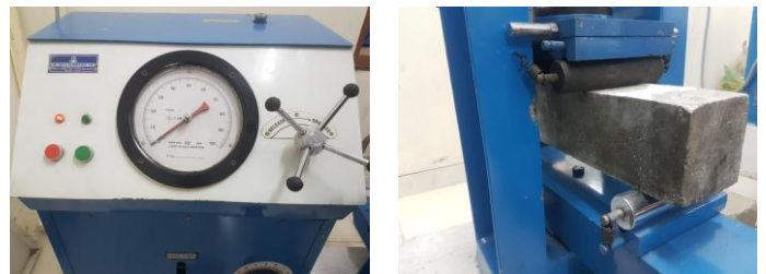
Fig 4: Flexural Strength Testing Machine and Specimen Placed in Machine
