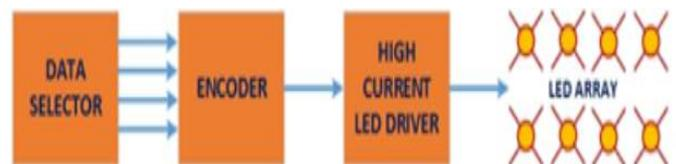
Fig -1: Block Diagram of Transmitter
