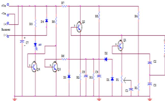
Figure -1: Circuit Diagram of a Metal Detector
