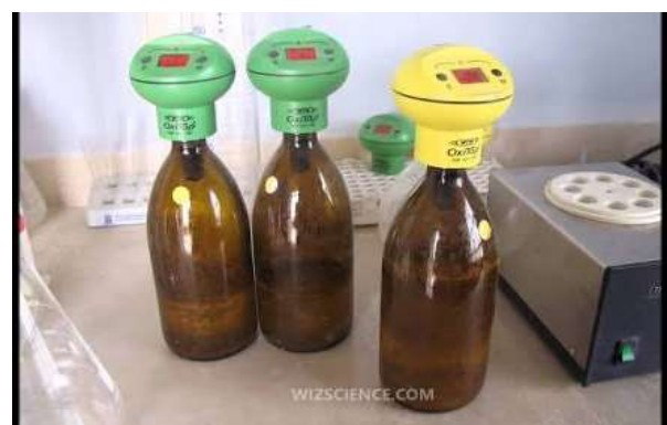
Fig - 3: Experimental setup for BOD
