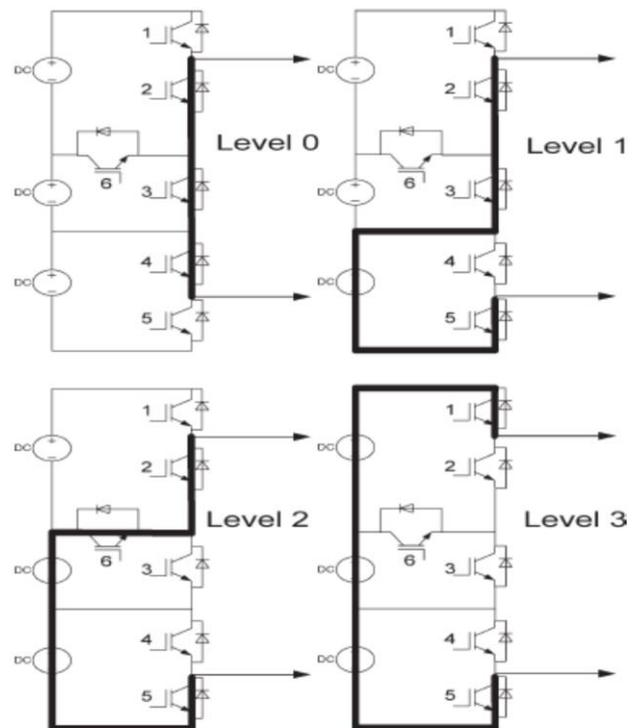
Fig -2: Switching sequence for various level generation
