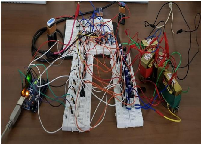
**Fig-4:** Seven level reversing voltage inverter prototype
