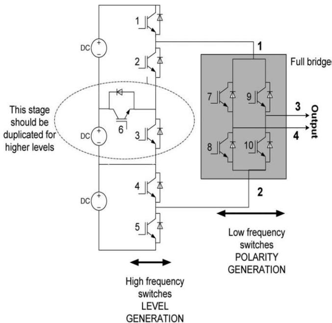
Fig -1: Schematic diagram of seven level inverter
