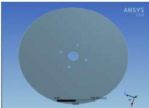
Fig2: Ansys model of furrow disc opener
