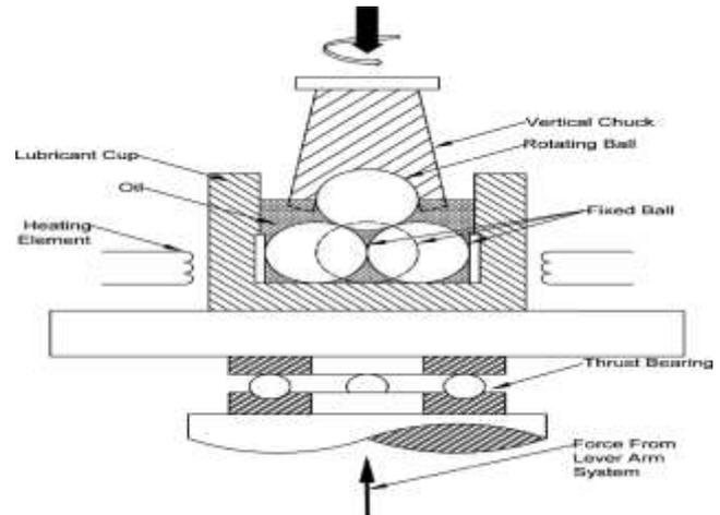
Fig. 1 Schematic diagram of four ball tester
