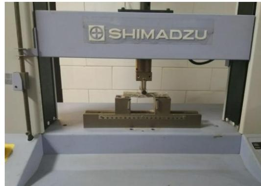
**Fig-2: UTM with Flexural test arrangement**
