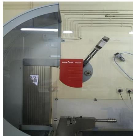
**Fig-3: Pendulum izod impact testing machine**
