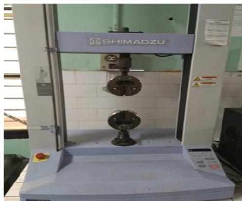
**Fig-1:** Universal Testing Machine
