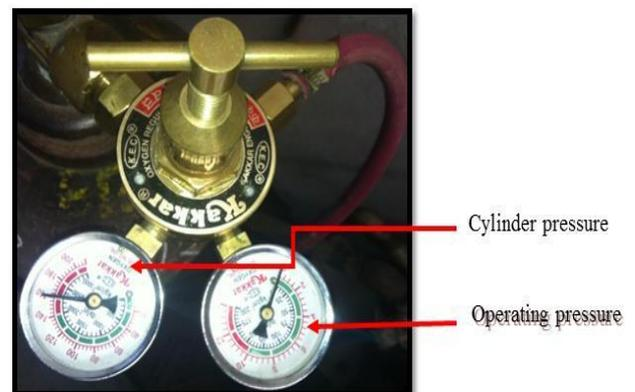
**Figure 3.3: Photograph of Oxygen Gas Cylinder Regulator**
