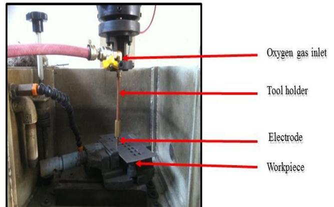
**Figure 3.2: Experimental Setup of Dry EDM**
