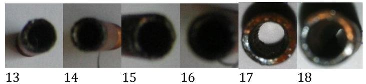
Figure 4.2: Photograph of Collection of Electrodes after Dry EDM Process
