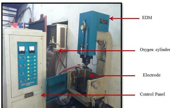
**Figure 3.1: Photograph of S20S EDM Machine**
