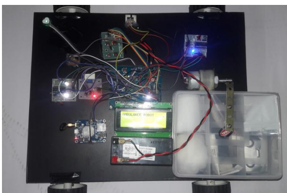
Figure 5- Experimental model of Robotic ambulance
