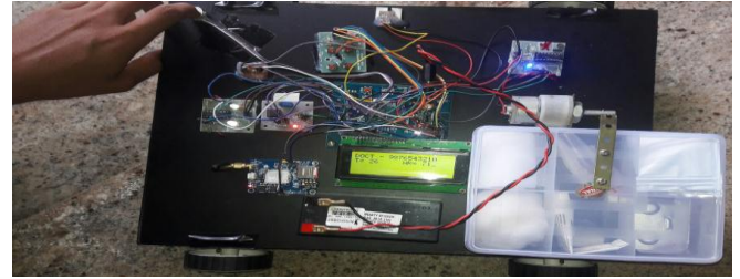
Figure 6- Temp and heartrate is being displayed on lcd
