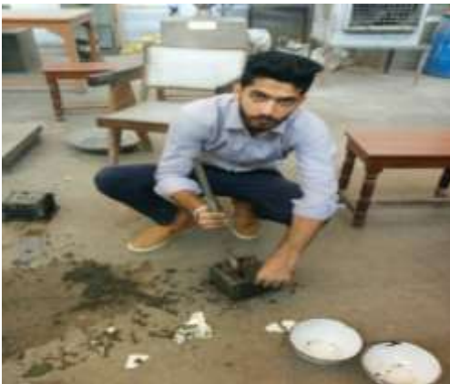
CUBE BEING FILLED
