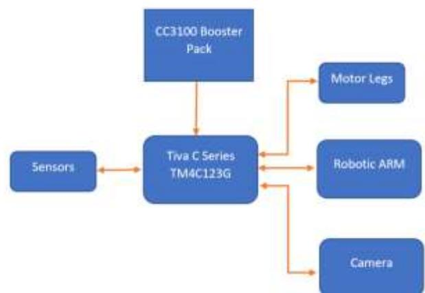
Fig -1: Block Diagram (Receiver Block)
