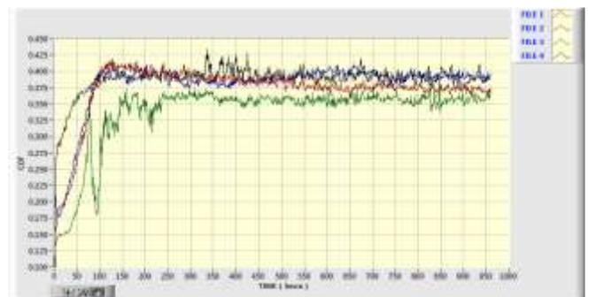
Fig-8: Variation of COF v/ s time with the addition of hBN Reinforcement under 20N load.
