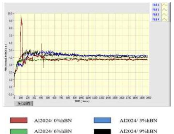
Fig -4: Variation of friction force v/ s time with the addition of hBN Reinforcement under 10N.
