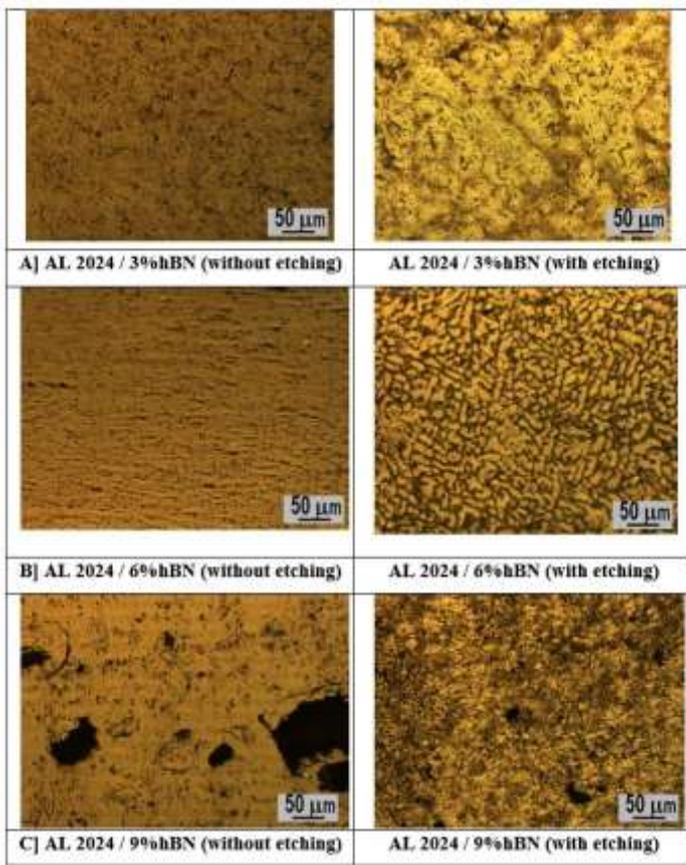
Fig -2: Optical micrographs of MMCs
