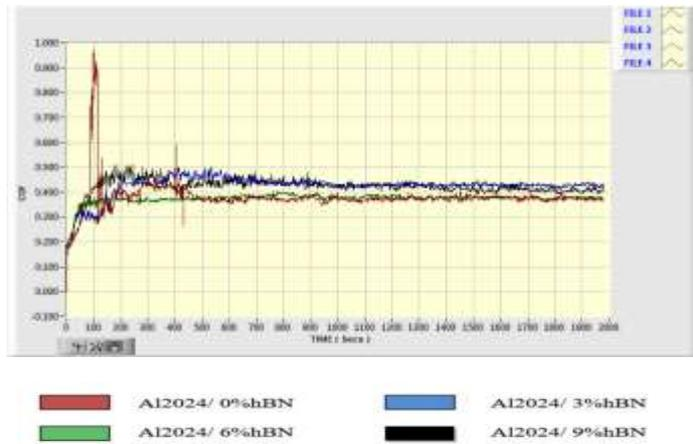
Fig-5: Variation of COF v/ s time with the addition of hBN Reinforcement under 10N load.
