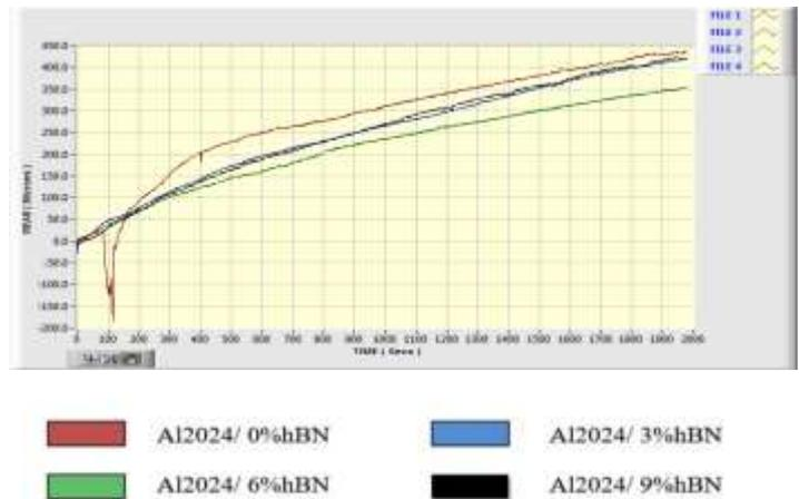
Fig -3: Variation of wear v/ s time with the addition of hBN Reinforcement under 10N load.
