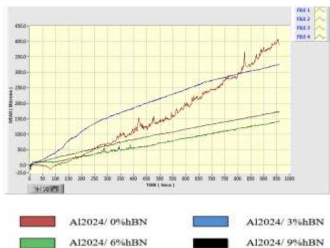
Fig-6: Variation of wear v/ s time with the addition of hBN Reinforcement under 20N load and 0.5m/s velocity.
