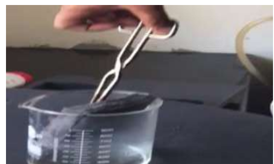
Fig 1 Treatment of sponge after heating the HCL solution
