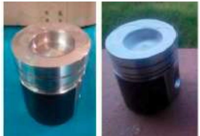
Fig -1: Sample of thermal barrier coated piston head is shown
