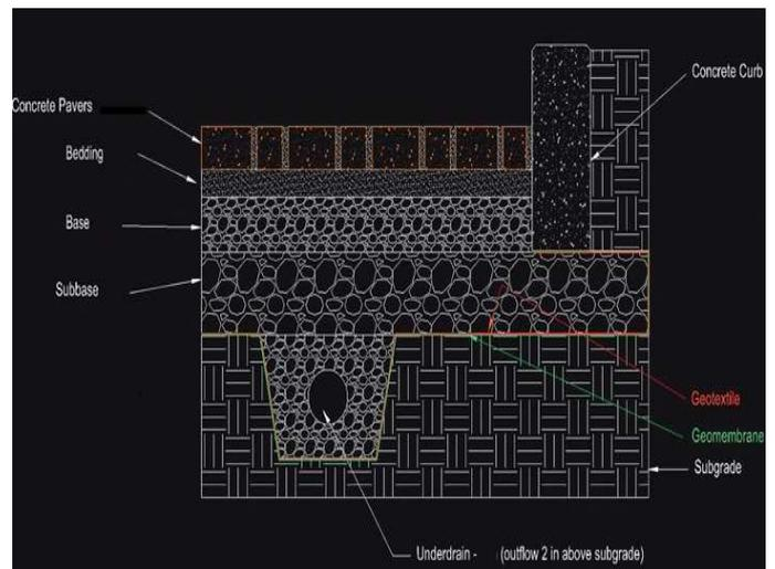
Fig:1 Typical Layers in Pervious Paving
