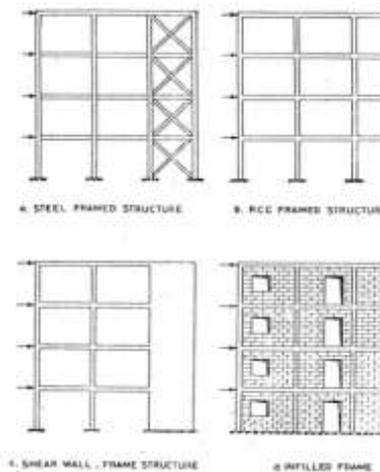
Fig-1: Lateral load resisting structures
