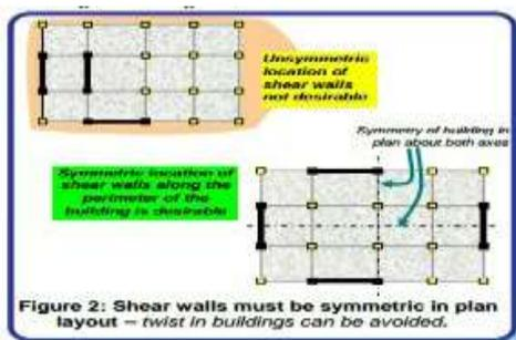
Figure 2: Shear walls must be symmetric in plan layout – twist in buildings can be avoided.
