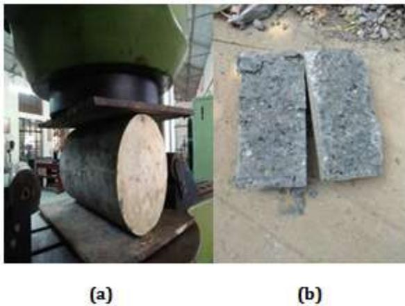
**Fig 6 (a) Split tensile test (b) Test specimen**
