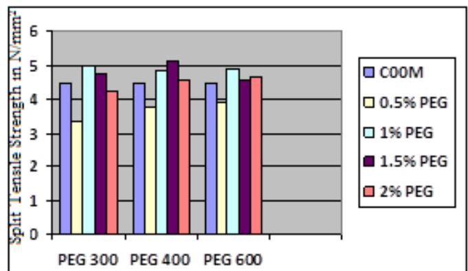
**Fig 6. Effect of self-curing agents on 7<sup>th</sup> day Split Tensile strength of concrete**
