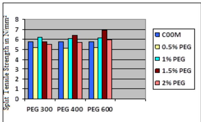
**Fig 7. Effect of self-curing agents on 28<sup>th</sup> day Split Tensile strength of concrete**
