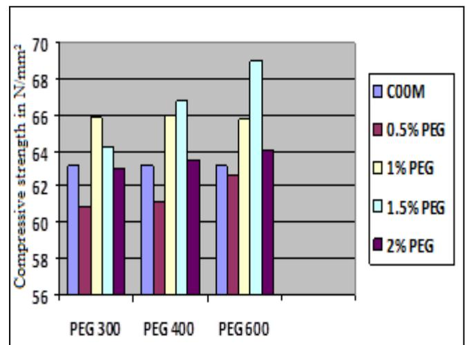
Fig 5. Effect of self-curing agents on 28<sup>th</sup> day Compressive Strength of concrete
