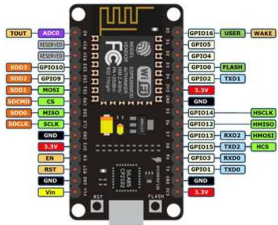
Fig 1: ESPNODEMCU pin diagram
