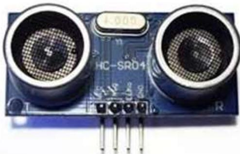
Fig 3: HC-SR04 Ultrasonic Sensors
