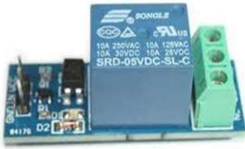
Fig 2: Single Channel Relay Switch
