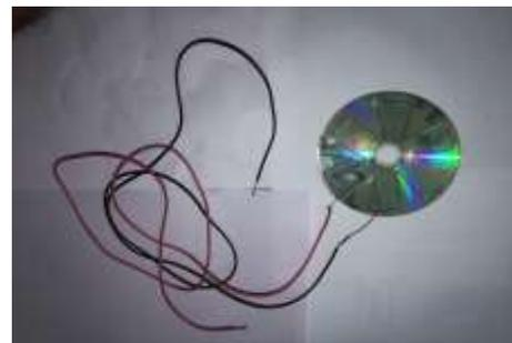
**Fig. no. 1 :** Bonding between CD & copper wire
