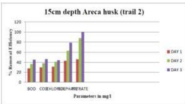
Removal efficiency using 15cm Areca husk filter bed
