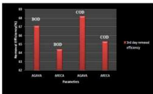
Comparison of BOD and COD Removal Efficiency (30 cm depth)
