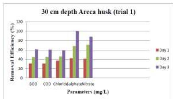
Removal efficiency using 30cm Areca husk filter bed
