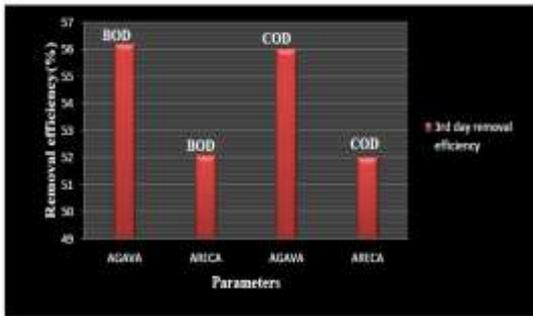
Comparison of BOD and COD Removal Efficiency (15cm depth)
