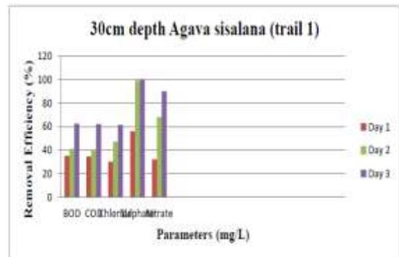
Removal efficiency using 30cm Agava sisalana filter bed
