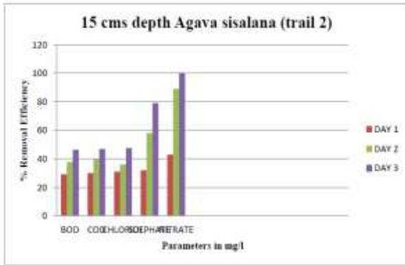
Removal efficiency using 15cm Agava sisalana filter bed
