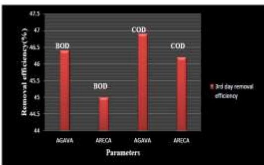
Comparison of BOD and COD Removal Efficiency (15cm depth)
