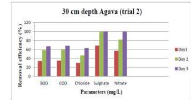
Removal efficiency using 30cm Agava sisalana filter bed
