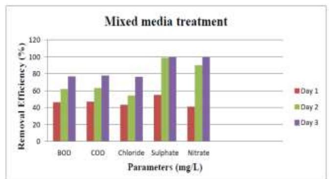
Removal efficiency using combined filter beds.
