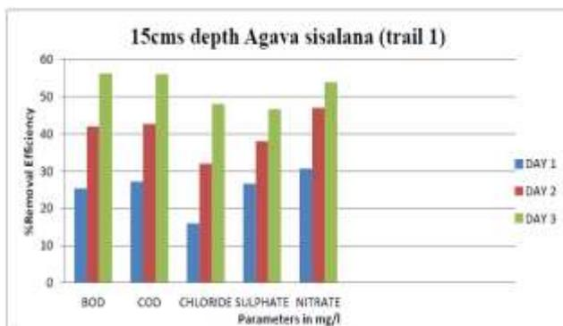
Removal efficiency using 15cm Agava sisalana filter bed
