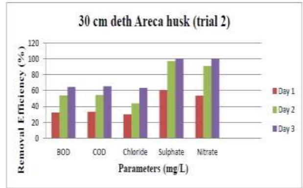
Removal efficiency using 30cm Areca husk filter bed
