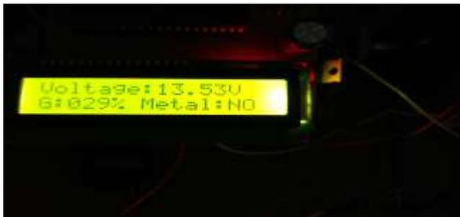
Figure 4. Voltage, Gas, Metal detection display
