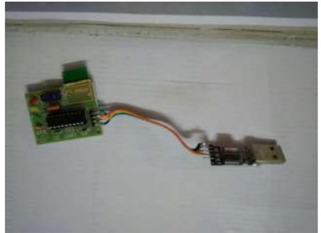
**Figure 2. RF Transceiver**
