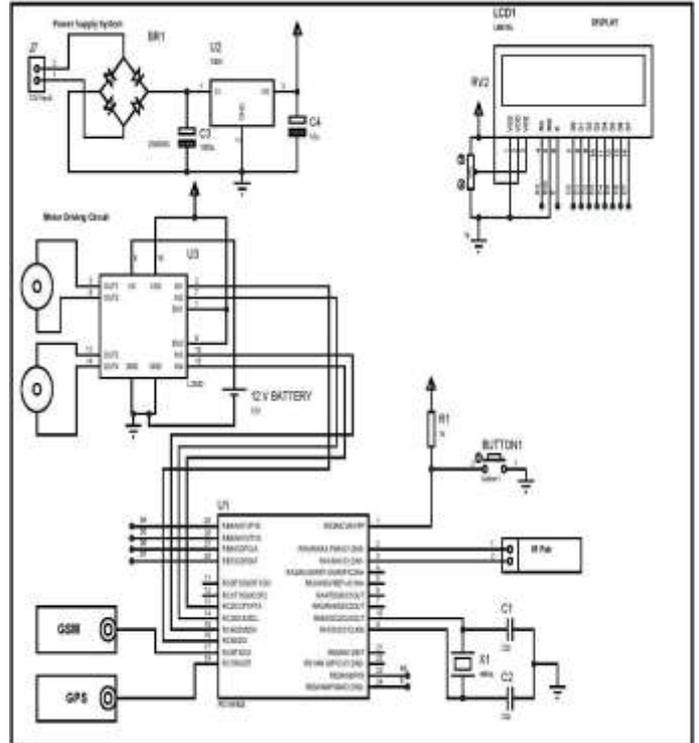
Fig -2: Circuit Diagram of Enhanced Railway Track Security System
