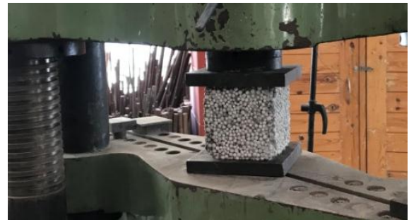
Fig -8: Compressive Strength Test
