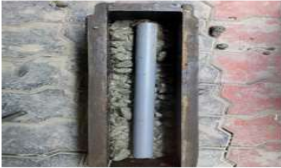
Fig 1: Beam with pipe
