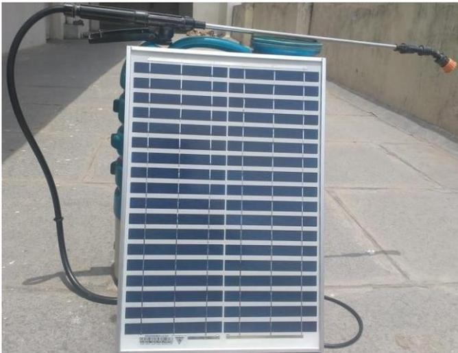
**Fig.4: Fabricated solar pesticide sprayer**
