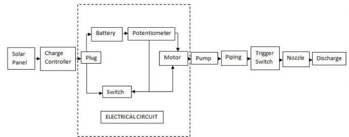
Fig. 5.1 Block Diagram of Spraying System.
