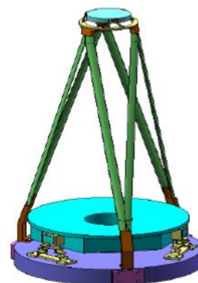
Fig. 4 3D structural model for deployable telescope
