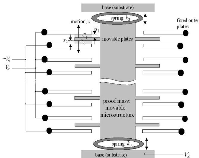
**Fig -4:** Accelerometer structure. Proof mass is attached through springs ( $k_s$ : spring constant) at substrate.
