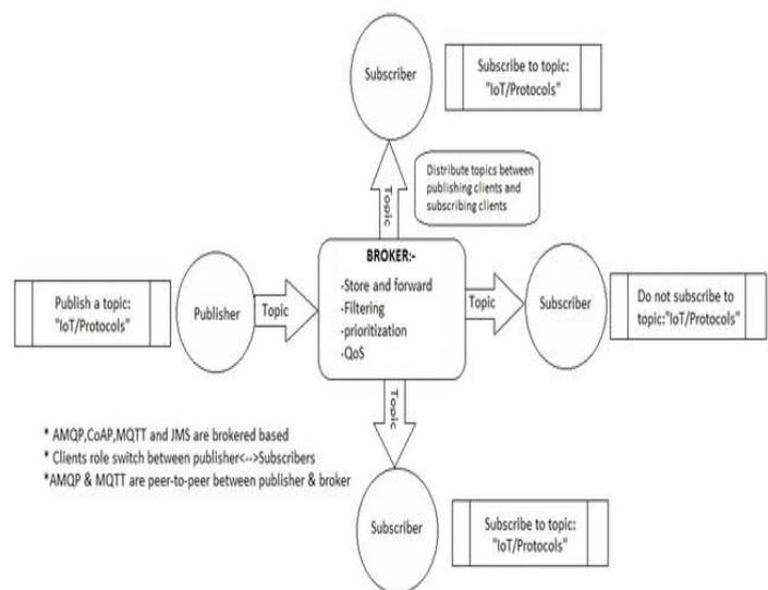
**Fig -5:** MQTT Broker based architecture
