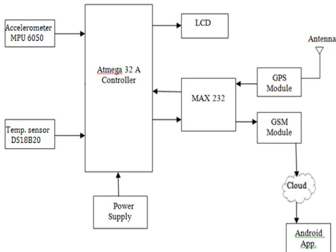
Fig -1: Block diagram of animal monitoring system
