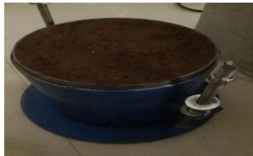
Fig -3: CBR Test Mould
