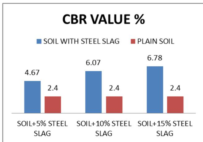
**Chart -5:** CBR value for plain and various steel slag mixed BC soil sample
