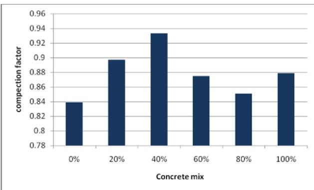
**Fig5: Compacting factor test results (0.50w/c)**
