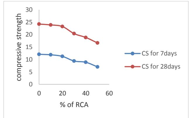
**Fig:7 Recycled coarse aggregate are used in different percentages of concrete the Compressive strength of concrete is gradually decreases at 7days and 28days**
