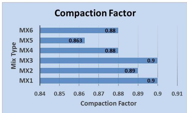
**Fig:6 Different Types of Concrete Mix V/S Compaction Factor**
