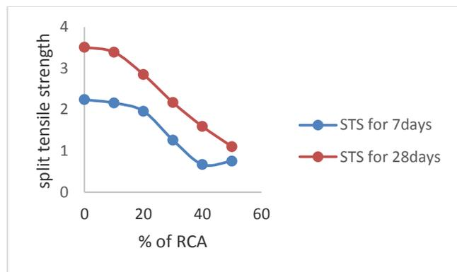
**Fig:8 recycled coarse aggregate are used in different percentages of concrete the Split tensile strength of concrete is gradually decreases at 7days and 28days**
