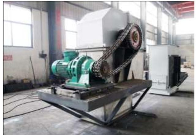
**Fig 3.1** Paper on Bucket Elevator Duplex chain Drive
