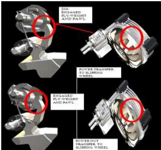
**Figure 9:** Locking differential by centrifugal force <sup>[12]</sup>
