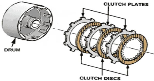
Figure 3: Locking differential by clutch pack [8]
