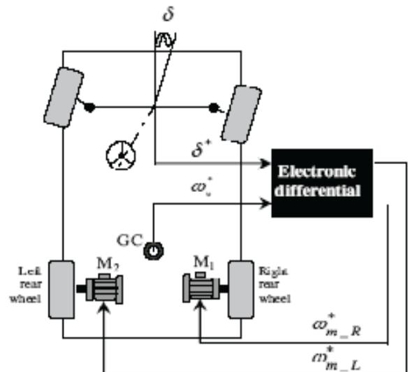
Figure 5: Electronic controlled differential [5]
