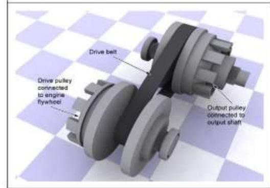
Figure 7: Continuous variable transmission differential [1]
