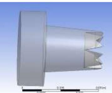
Fig-4: Three dimensional view of M Lobe chevron nozzle model
