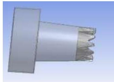
Fig-6: Three dimensional view of m lobe chevron with sinusoidal nozzle model
