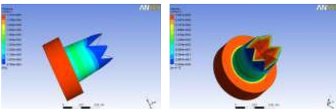
Fig-11 pressure distribution of chevron asymmetric nozzle model
