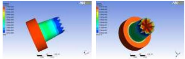
Fig-13 pressure distribution of M lobe chevron nozzle model
