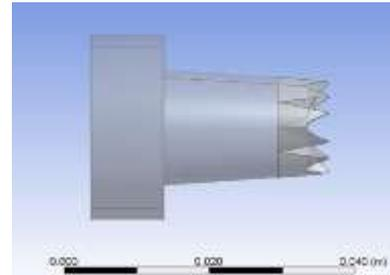
Fig-5: Three dimensional view of M lobe chevron with c curve model
