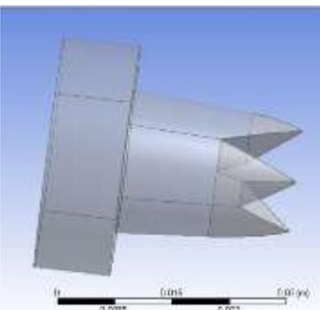
Fig-3: Three dimensional view of asymmetric chevron nozzle model.
