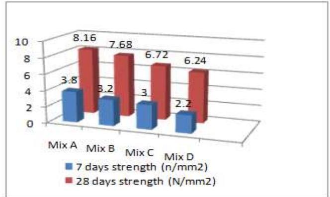
**Chart -2:** Comparison of Flexural Strength of Different Mix
