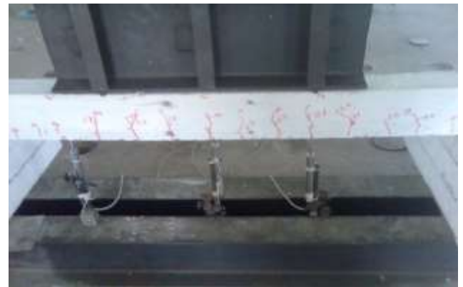
Fig 3.6 Testing of Beam Specimen
